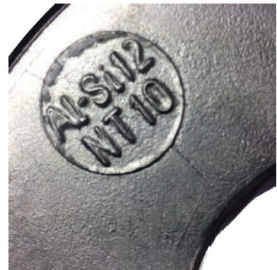
Surface quality using centrifugal casting. With permanent moulds, a surface quality of 20 - 120 RMS can be reached
