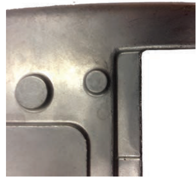
Surface quality of pressure die casting. With permanent moulds, a surface quality of 20 - 120 RMS can be reached
