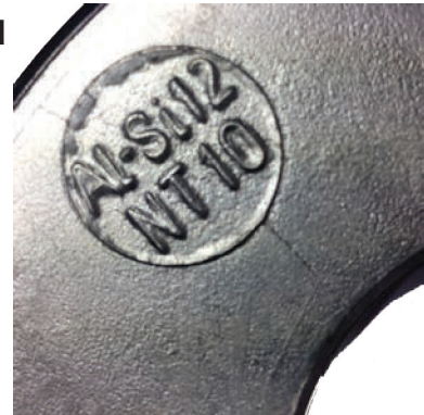
Surface quality using gravity die casting. With permanent moulds, a surface quality of 20 - 120 RMS can be reached
